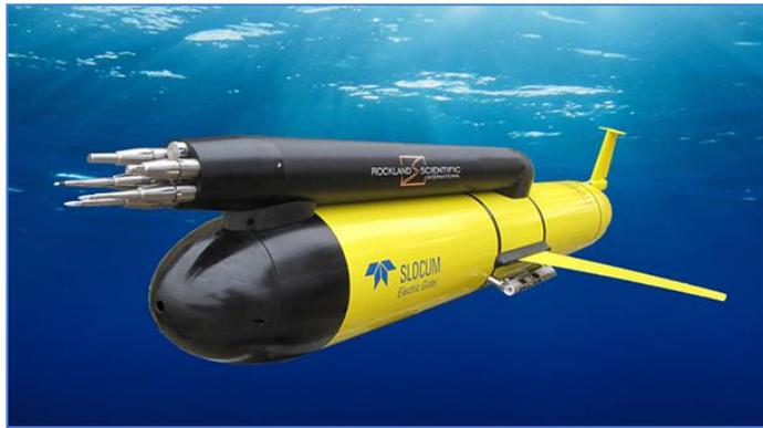
Autonomous underwater vehicle, operating along vertical sections to monitor the water column up to 1000 m depth. It provides vertical profiles of hydrological properties and turbulence through continuous cycles of immersion-emersion. The system was acquired by CNR in 2014 as part of the project EUROFLEETS.
